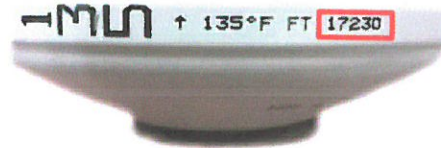
Figure 2: Location of manufacturing date code on detector. (August 18, 2017) Format: (YY = last two characters of calendar year, DDD = Ordinal/Julian number of the day of the calendar year)
